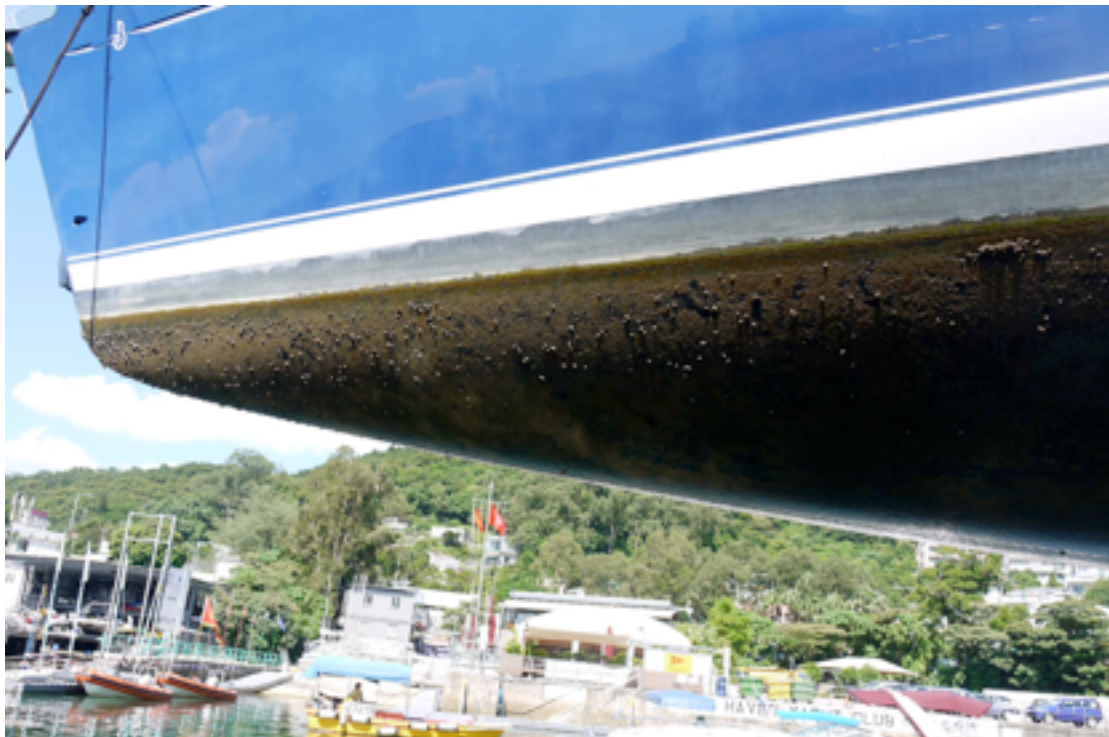
6. ANOTHER VIEW OF THE FORWARD HULL AND MINIMAL BARNACLE BUILDUP.
