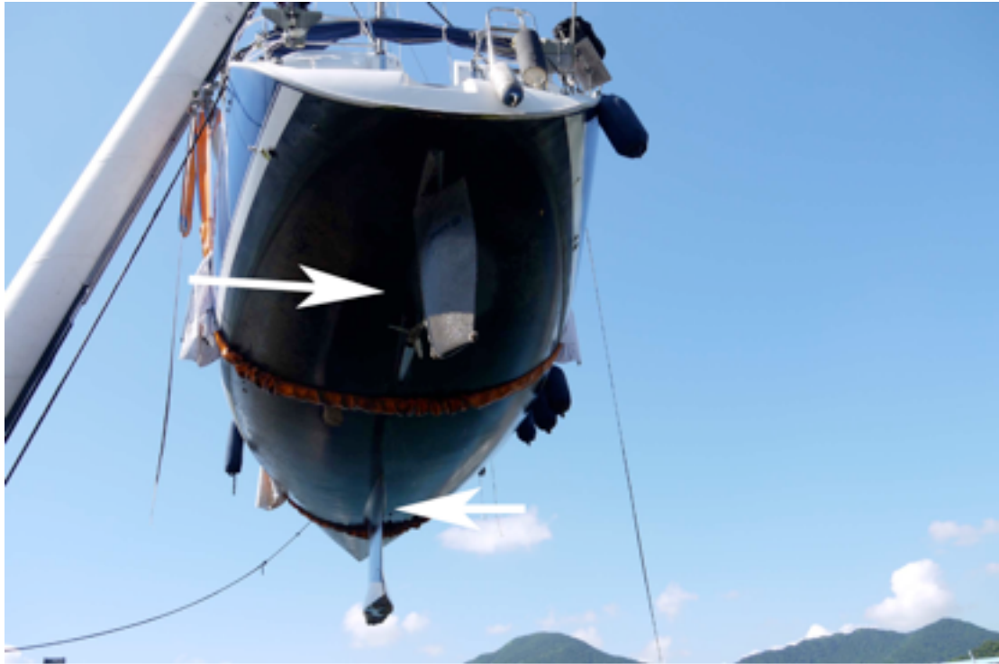
1. LOCATION OF TRANSDUCERS AND CONDITION OF HULL WHEN LIFTED AFTER 20 MONTHS.
