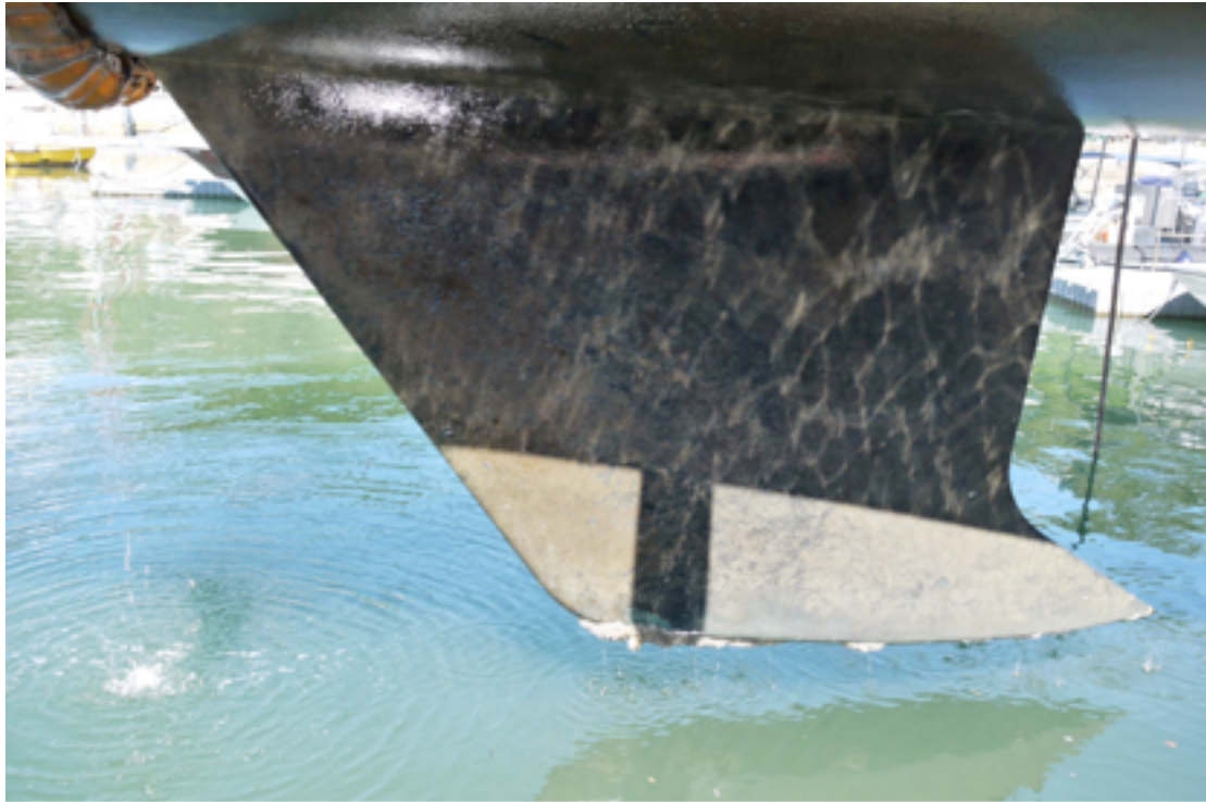
5. KEEL. FOULING POSSIBLY DUE TO 'BUMPING' THE BOTTOM DURING LOW TIDES.
